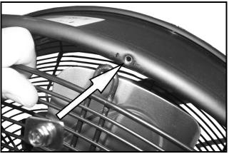
Wipe the fan blades with dry cloth and remove any dust from the motor assembly with a soft paintbrush, vacuum cleaner or jet of compressed air.
